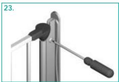
Tighten 3 sets of assembly screws and nuts.
