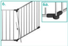
To remove vertical bar, lift up on bar (5), while sliding it out of lower hinge groove (6a.). Pull bar down and out of cone (6.).
