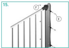
Insert 3 wall cover screws (E) through oblong holes in top, middle and bottom of assembly.
