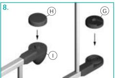
Depending on number of sections removed, you will end up with one of two configurations at the end of gate (diagram 8 or 9).
