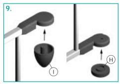
Remove hinge cap (H) from bottom of original end section. A screwdriver may be needed to pry it off. Place under bottom hinge. Remove plastic cone from under top hinge of original end section. Install cone (I) under top hinge of new end section.
